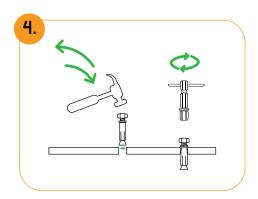
Hammer down the nails and screw it till it holds.
