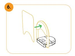
Fix the QR code plate to the Bouncer with double-sided tape or screws.
