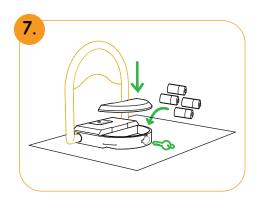
Plug the batteries. Close and lock the battery compartment and the device lid.
