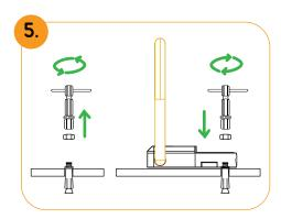
Unscrew the bolts and place the device then screw the bolts again.
